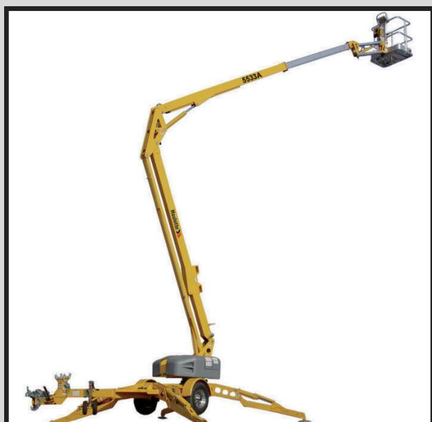
Haulotte 5533 A 55 Ft Electric Articulating Towable Boom Lift can be towed by a standard half-ton pickup truck - No commercial driver's license needed. Superior combination of industry leading capacity and outreach. Hydraulic outriggers and automatic leveling allow operation in under 30 seconds.
