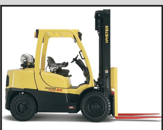
8,000 lb capacity with a 24-inch load center, featuring pneumatic tires, and solid dimensions like a roughly 7-8 ft lowered mast height and around 9-10 ft max fork height, built for high-intensity indoor/outdoor work with good gradeability (around 30%)
