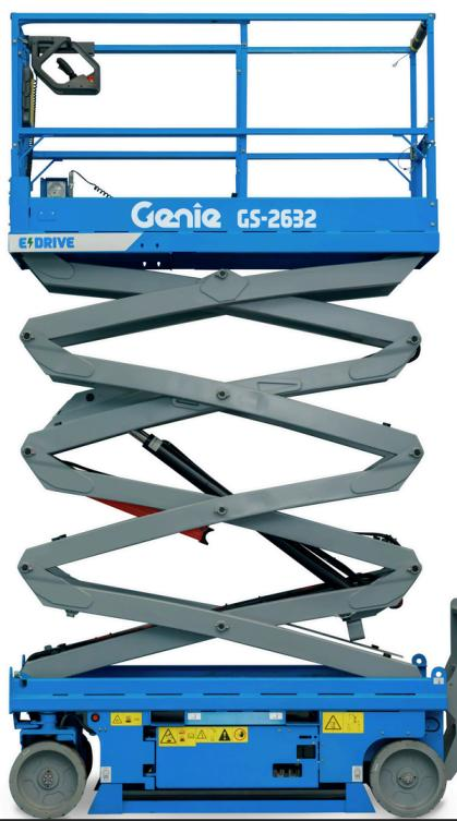
The Genie GS-2632 E-Drive self-propelled electric scissor lift is ideal for maneuvering in tight spaces, making it the right choice for indoor and outdoor construction, maintenance and installation applications with firm, level surfaces.
