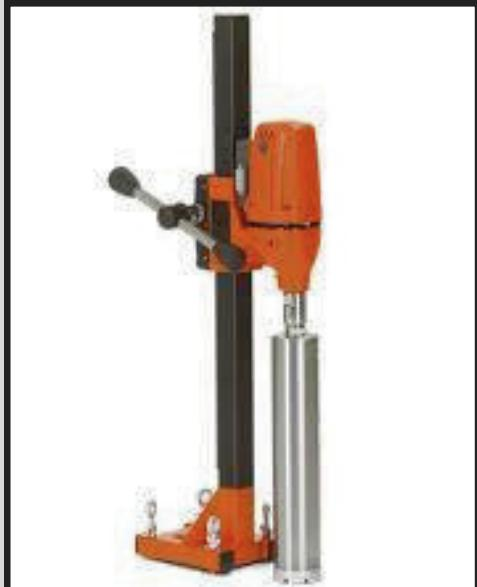
DMS 240 is an electric drill motor and stand system for a wide variety of core drilling applications. An ideal system for medium core drilling in walls, floors and roofs up to 10 in. diameter. The stand is easy to tilt, and the back support provides reliable and stable angle drilling, saving you setup time and body stress. This system can be used for ventilation, plumbing waste evacuation pipes, barriers and road signs.
